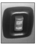
Press and release the rear of the switch and the glass panel will open to the vent position.
